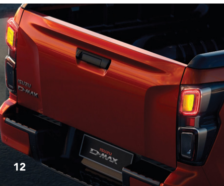
12 Emergency Stop Signal (ESS) In emergency situations, warning lights are activated to indicate that the vehicle is braking rapidly.
